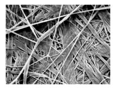
DuPont<sup>™</sup> Tyvek<sup>®</sup> is a nonwoven, nonperforated sheet of spunbonded high-density polyethylene (HDPE) with microscopic pores large enough for moisture vapor to pass through, but small enough to resist air infiltration and water intrusion. The unique combination of properties – air infiltration resistance, bulk water resistance and vapor permeability help protect a home from the elements, improve energy efficiency and prevent moisture from accumulating in walls.
