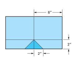
6" **FlexWrap**™ (for greater than 4" recesses, single stud framing)
