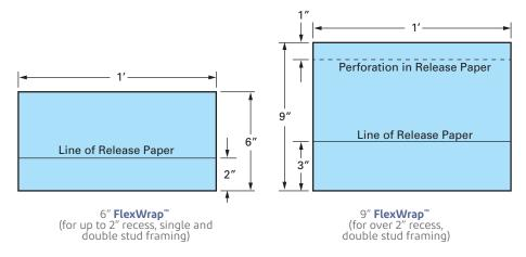
The following photos show the fabricated Recessed Window Corners for a recess that is up to 2" deep with double stud window framing using 6" **FlexWrap**™ (left) and a recess that is 4" deep with double stud window framing using 9" **FlexWrap**™ (right).
