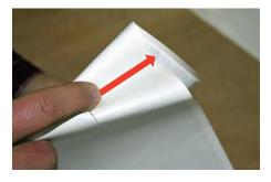
5. Create Corner Fold. On the reverse side of the **FlexWrap**™, starting at the intersection of CREASE A and CREASE B, fold along CREASE B going out towards edge of narrow release paper.
