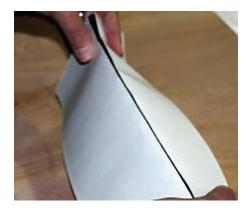
2. Create Horizontal CREASE A. Fold **FlexWrap**™ at release paper to break perforations and create crease.
