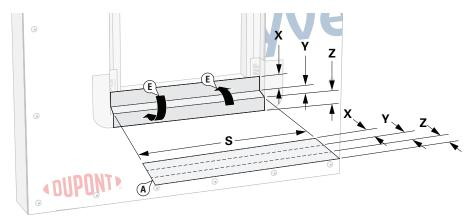
Table 1: Sill/Head Flashing for Shallow Recessed Flanged Window Condition
