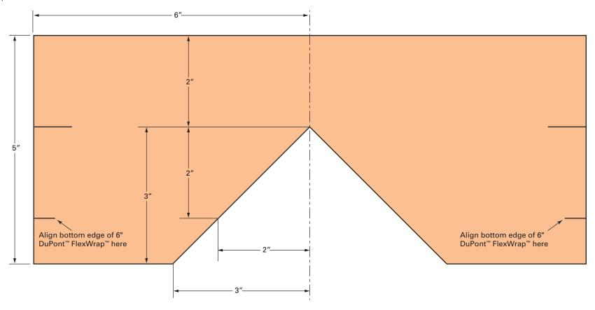
Align the bottom edge of 6" **DuPont™ FlexWrap™** with the the 2" marks (for up to 2" recess). Align the bottom edge of 9" **FlexWrap™** with the lower edge of the template (for recesses greater than 2").
