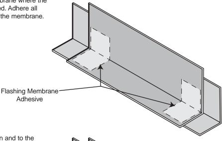
2. Mount the cloak on and to the membrane. Use firm hand pressure to assure a secure attachment.
